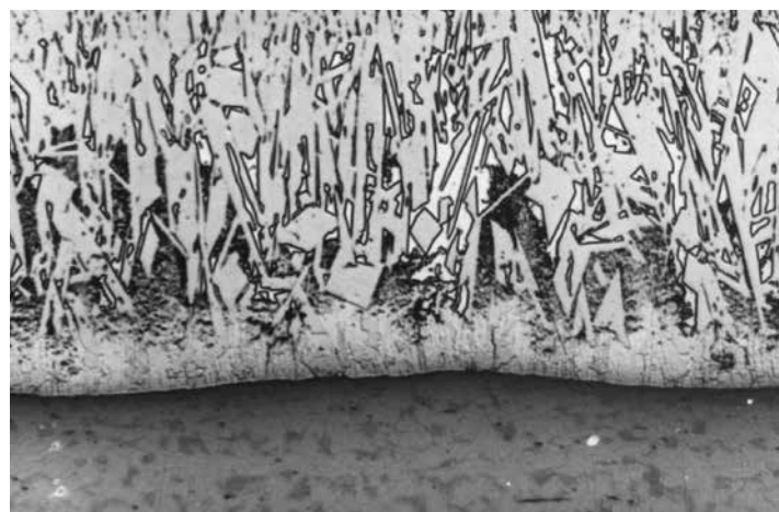
Fig 3. Microstructure of a thick coating obtained on a reactive steel
