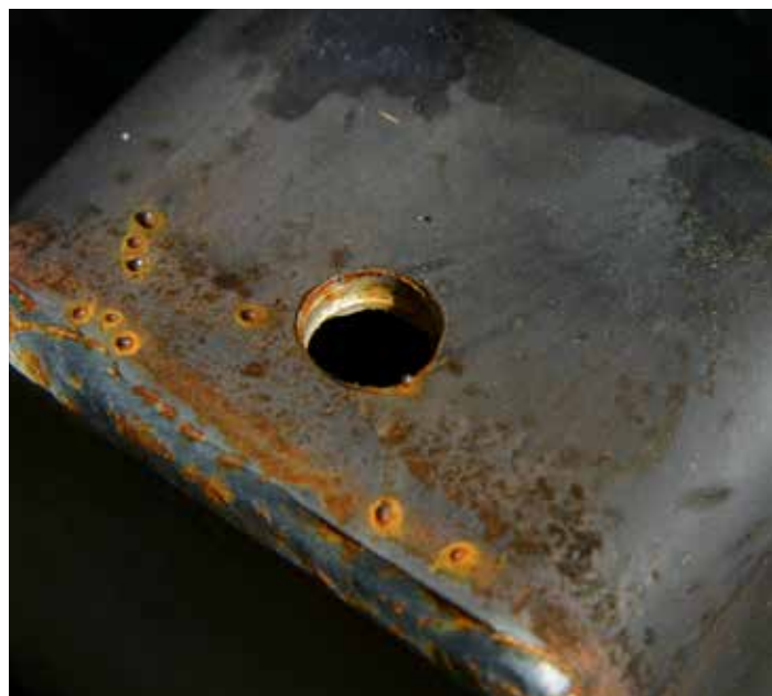
Fig 1. Weld spatter present on steel before galvanizing
